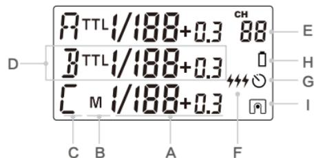
(A) Output Settings per Group in the M Mode; FEC Settings per Group in the TTL Mode
